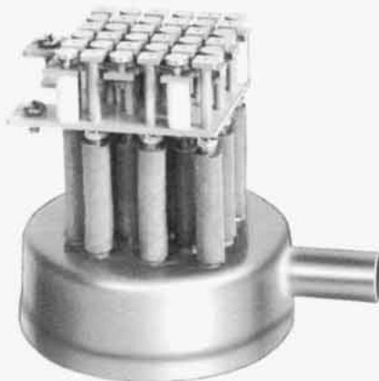
Figure 6. Grid electrode holder for measuring mica in a plane parallel to the cleavage plane. (Courtesy of Bell Telephone Laboratories and American Society for Testing Materials. From ASTM Designation: D748-54T. Reprinted with permission.)
