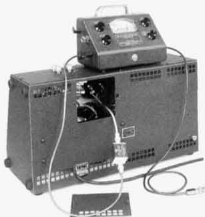
Figure 8. Q Meter, Type 260-A connected to RF Voltage Standard, Type 245-B.
